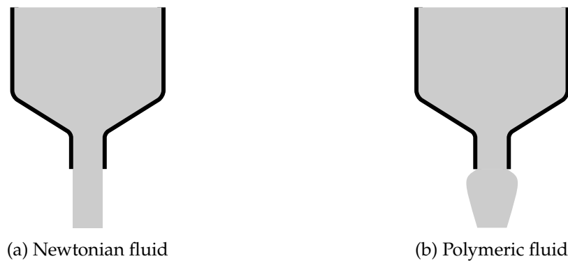
Figure 1.3. Visualization of the extrudate swell or Barus effect. Fluids of different type are pushed through a tube with a contracted exit.
