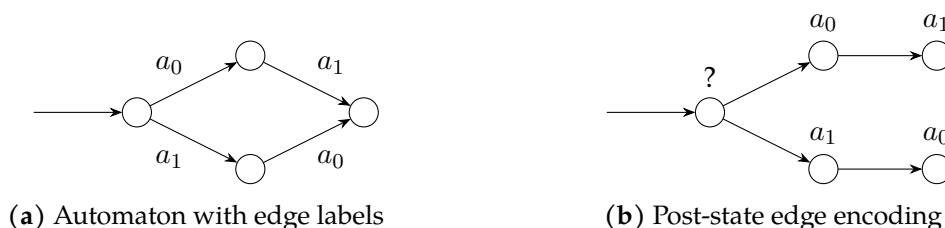
Figure 4.2: The employed post-state label encoding for Listing 4.1. Edge labels denoting the identifier of the respective action in the labeled transition system (LTS), as shown on the left, are moved into the edge target where their respective effect unfolds, as shown on the right. Note that we regard those atoms induced by the post-state edge encoding as immaterial in our calculations.
